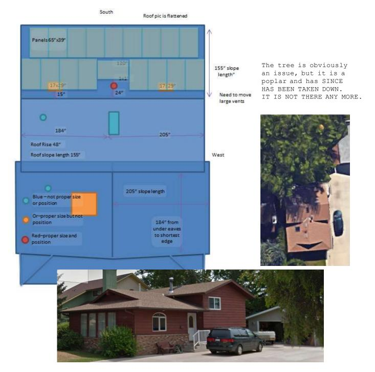
The cost of electricity at my fixed rate is CperKwH= 5.999 The solar panels sizes are l= 65 in w= 39 in w. area The main roof size: lroof= 155 in wroof= 184 in+205 in wroof= 389 in
