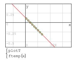
Efficiency factor of panels on Temperature - we assume 25deg C for Calgary
