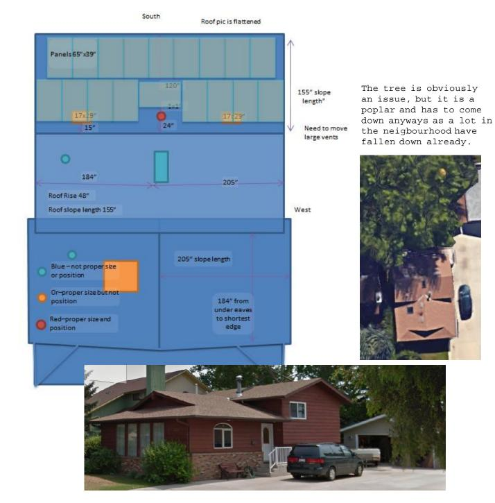
The cost of electricity at my fixed rate is CperKwH= 5.999 The solar panels sizes are l = 65 in w = 39 in w. area  $l \cdot w = 1.6355m^2$ The main roof size: lroof = 155 in wroof = 184 in + 205 in wroof = 389 in
